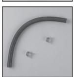
**FUEL LINE** 4, 6, 7.5 HP Vanguard™ (shut-off valve to carburetor) 4 mm OD x 220 mm (8-5/8") cut to fit Part No. 715126
